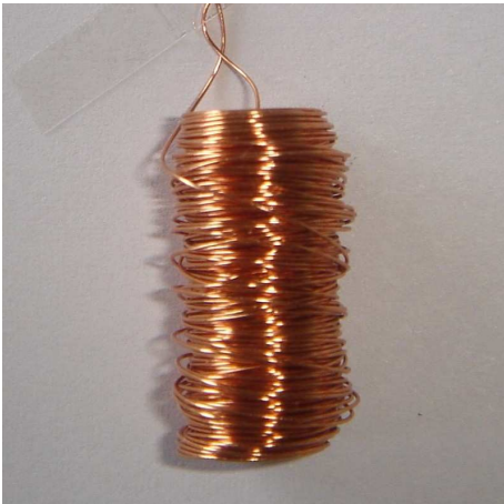
Ant 5) Coil, n=800, Di=3mm
