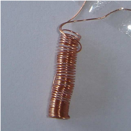
Ant 3) Coil, n=40, Di=3mm
