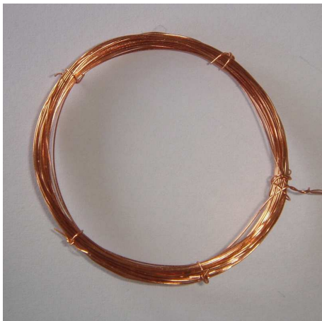
Ant 6) Coil, n=50, Di=30mm
