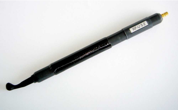
Pic 6: Near Field Probe
